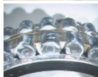
Photo. 6.2 Filling grease into cylindrical roller bearing
